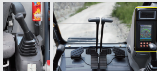
●高度灵敏的先导手柄 Sensitive joystick
